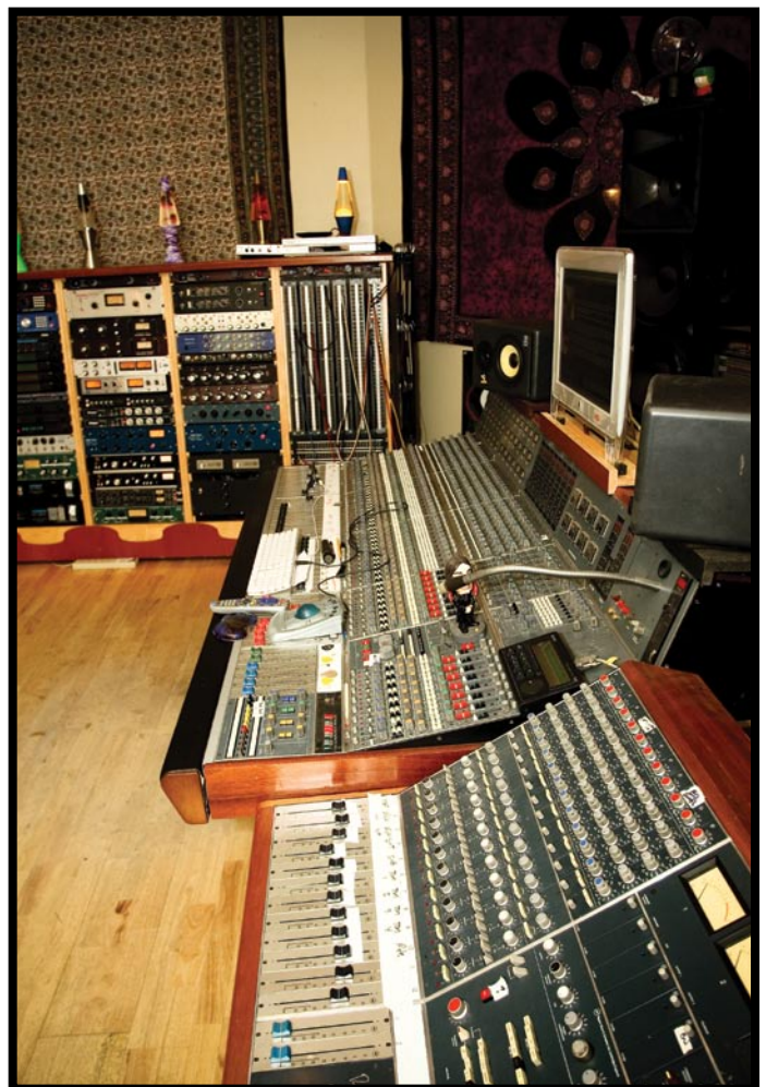
ABOVE: Studio B The Mixing Studio featuring SSL 6064 E G+ TR HD-3 with 64 outs @192, Custom Westlake Monitors, and ATR 102 1" Mixing deck. RIGHT: Studio A Control Room with Neve (discrete) Console with (36) 33114 EQ/pres (1081s) and (8) 33314A (2254) Neve Compressors, and Neve Melbourne 12-channel discrete sidecar with 3114 EQ/pres.
